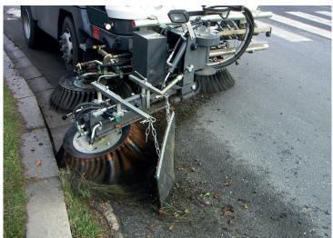
*N.B.* When ordering this option the option: Gutter brush angle adjustment should be reconsidered since the third brush is excellent for cleaning gutters.
